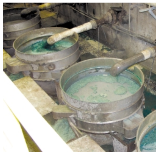
Photo 5: Sweco Screens remove solids from wastewater
