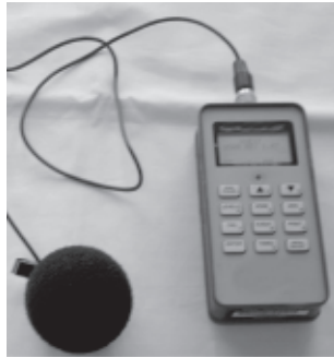
The American National Standard Institute ANSI S1.25 contains specifications for a noise dose meter. Slow time-weighted sound pressure is integrated with 5-db exchange rate in accordance with U.S. OSHA regulations 3
