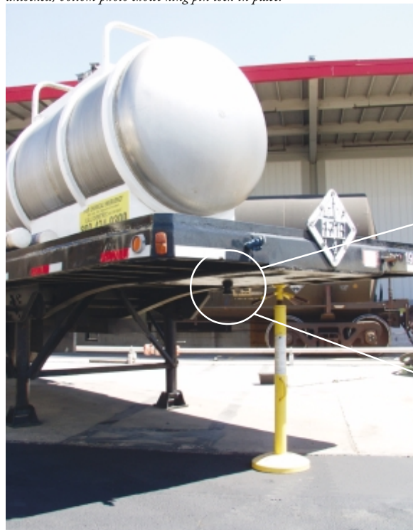
Photo below shows position of king pin. Below, right: top photo shows king pin unlocked, bottom photo shows king pin lock in place.
