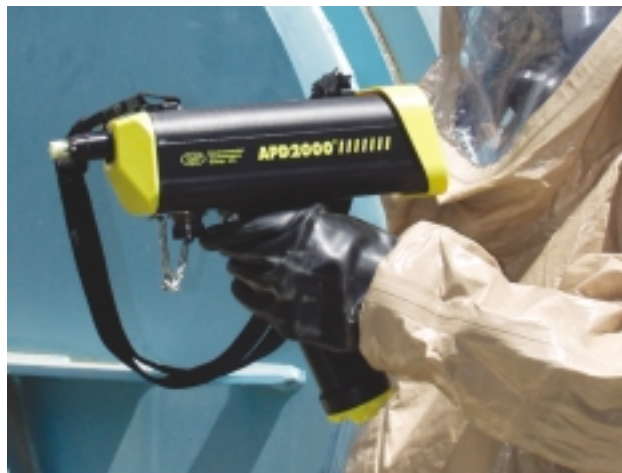
The ADP2000, an advanced Portable Chemical Agent Meter, can detect nerve agents, mace, and pepper spray. See paragraph, center right, next page.
